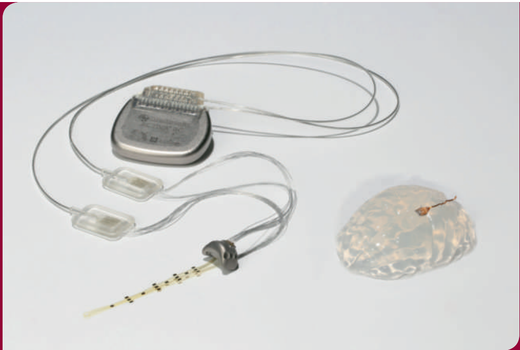
Some elements of the brain-spine interface: A microarray of electrodes on a silicon model of a primate brain, a pulse generator and a spinal implant composed of 16 electrodes
